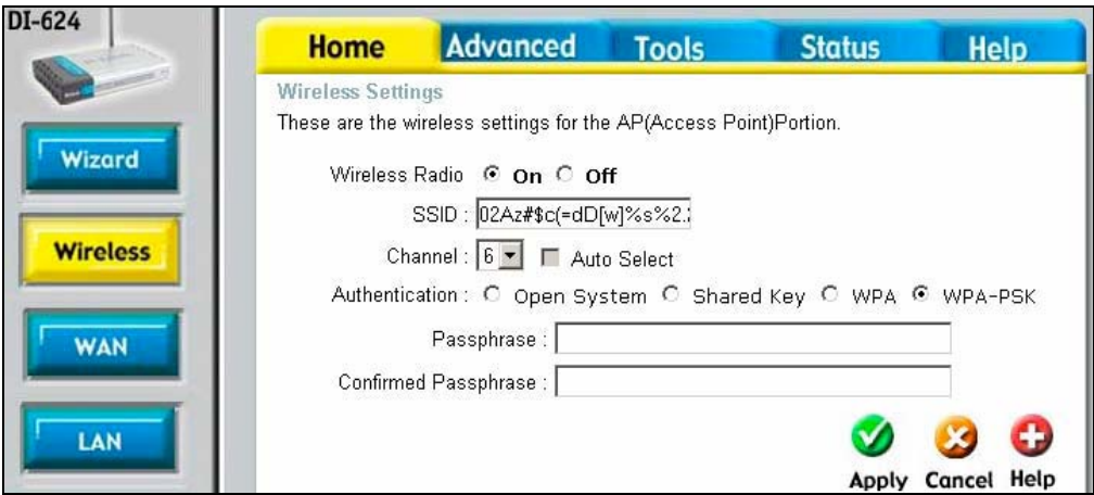
Figure 1-5. Dlink: Changing the SSID
